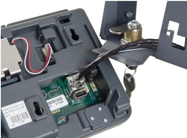
Figure 4: Clock with cables connected and partial wall mount
