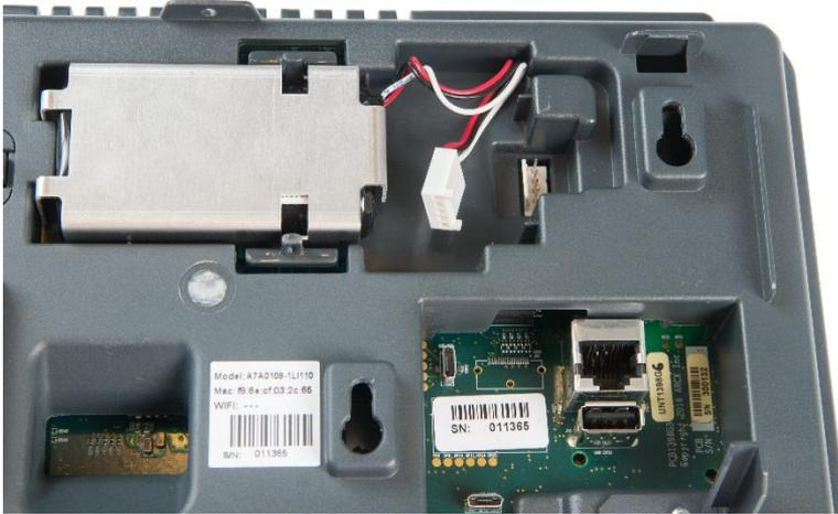
Clock with battery installed but not connected
