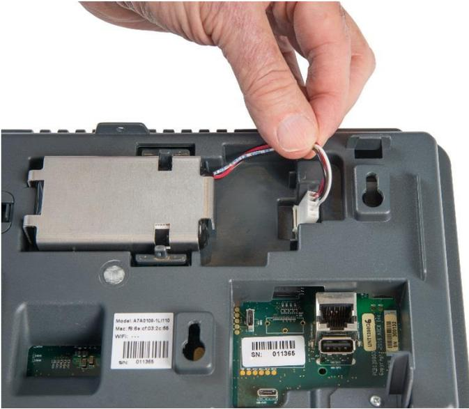
Inserting the wire connectors
